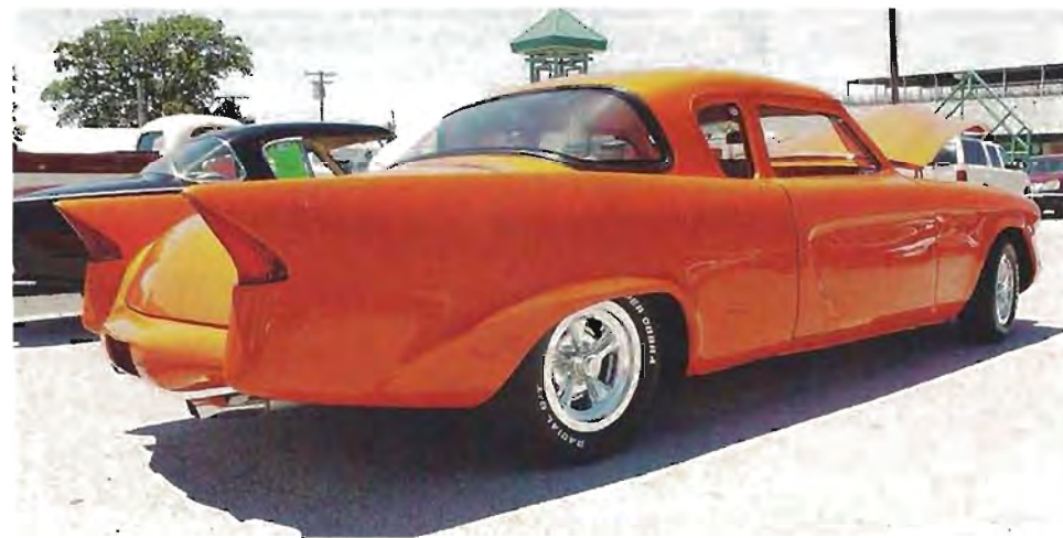
This custom combined the rear fender panel of a sedan or wagon with coupe styling. Cathedral style taillights accent fender fins.
